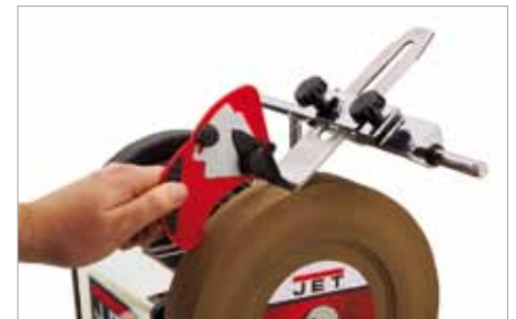
Controlled sharpening with angle guide
